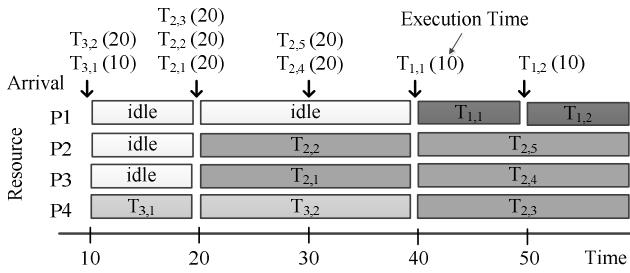
Fig. 1. An example of resource distribution on RCSM. The budgets of  $T_1$ ,  $T_2$ , and  $T_3$  are 1, 2, and 1, respectively.
