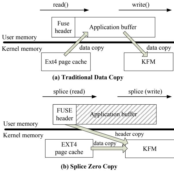
Fig. 2. Comparison between the traditional data copy and the zero copy under FUSE file system.
