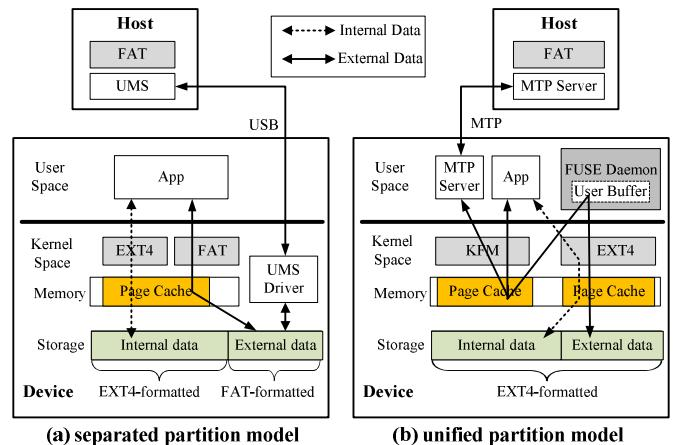
Fig. 1. Two models of externally-mountable partition at multimedia devices
