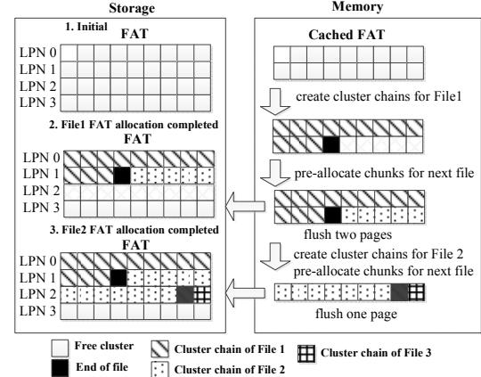
**Fig. 2 Page-aligned pre-allocation.**
